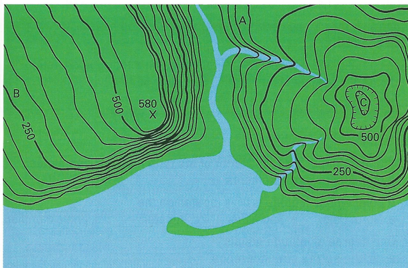
Figure 3–12. The features of the coastal valley shown in the diagram above are represented by contour lines on the topographic map below. What are the elevations at A and X?
