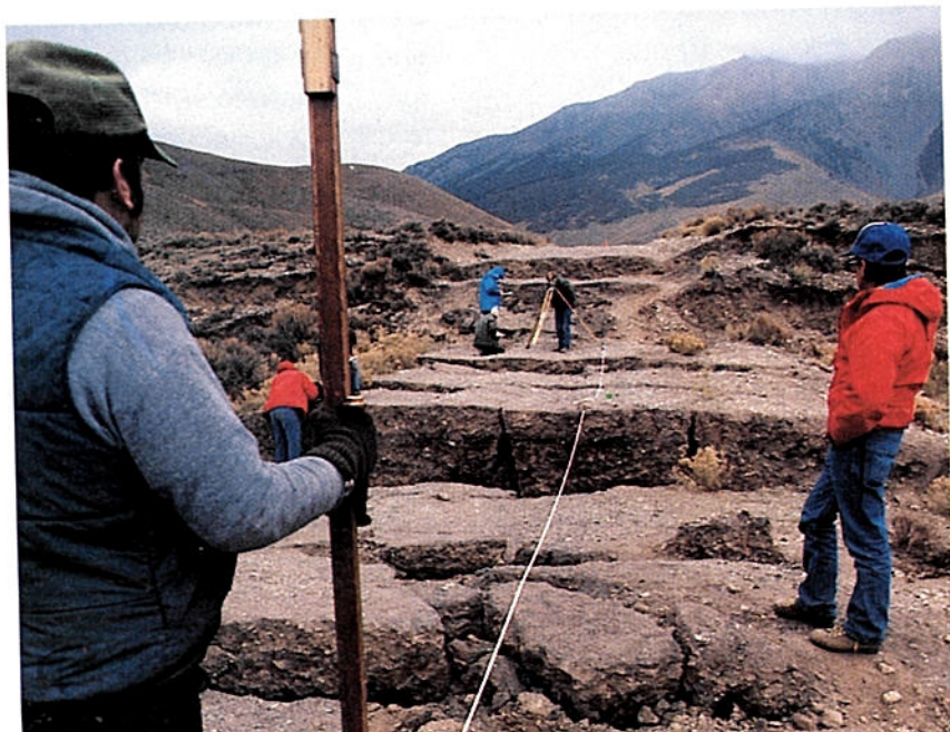
Figure 1-6. One means of gathering information is through careful measurement. In this photo, geologists are measuring a crack in the earth's surface caused by an earthquake.
